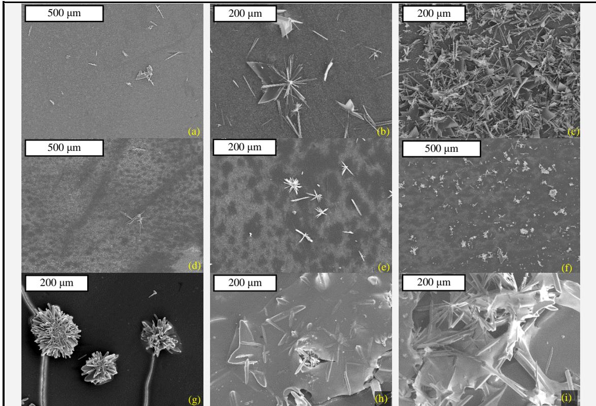
**Figure 1** SEM images of  $\text{CaSO}_4$  crystals deposited/developed on the desalination membrane. Scaling tests: a)  $S_w=1.30$ ; b)  $S_w=1.45$ ; c)  $S_w=1.57$ . Combined fouling/scaling tests: d)  $S_w=1.20$ , 2 mg/L SA; e)  $S_w=1.43$ , 2 mg/L SA; f)  $S_w=1.48$ , 2 mg/L SA; g)  $S_w=1.19$ , 10 mg/L SA; h)  $S_w=1.51$ , 10 mg/L SA; i)  $S_w=1.57$ , 10 mg/L SA
