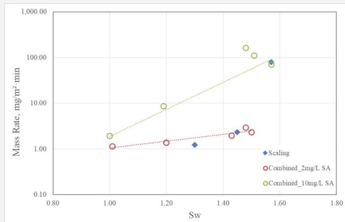
**Figure 2.** RO membrane scaling by calcium sulfate in the presence of SA; initial scale-mass deposition rate [ $\text{mg}/(\text{m}^2\text{min})$ ], versus membrane-surface supersaturation ratio  $S_w$ .
